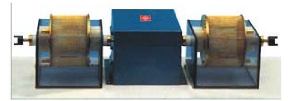
Figure 2.5: Slake durability apparatus
